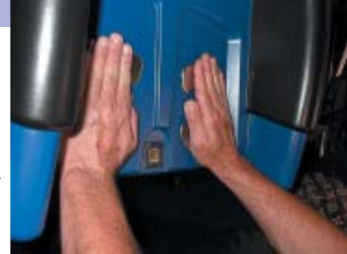
When students place their hands on the new Web-enabled kiosk's stainless steel plates, a slight electrical current passes from the left hand to the right hand, measuring lean body mass and weight, using bio-impedance, the measurement of the body's electric conductivity. Jennifer Larson photo
